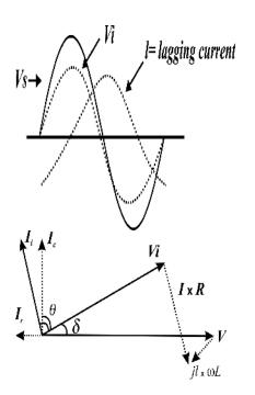
(b) Inductive mode Vs > Vi, If Vs > Vi then I is apper to be leading current since the magnitude of the current can be controlled continuously by adjustint Vi,the D-STATCOM will function as a capacitive reactance continuously controllable.
