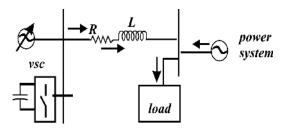
Fig. 2. Basic Building Blocks of the D-STATCOM.
