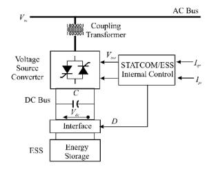
Fig. 1. Basic structure of D-STATCOM.
