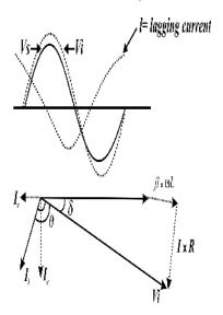
(c) Capacitive mode Vs < Vi. If Vi < Vs then I apper to be lagging current this mode. The D-STATCOM will function as a reactor whose inductive reactance is contineously controllable.
